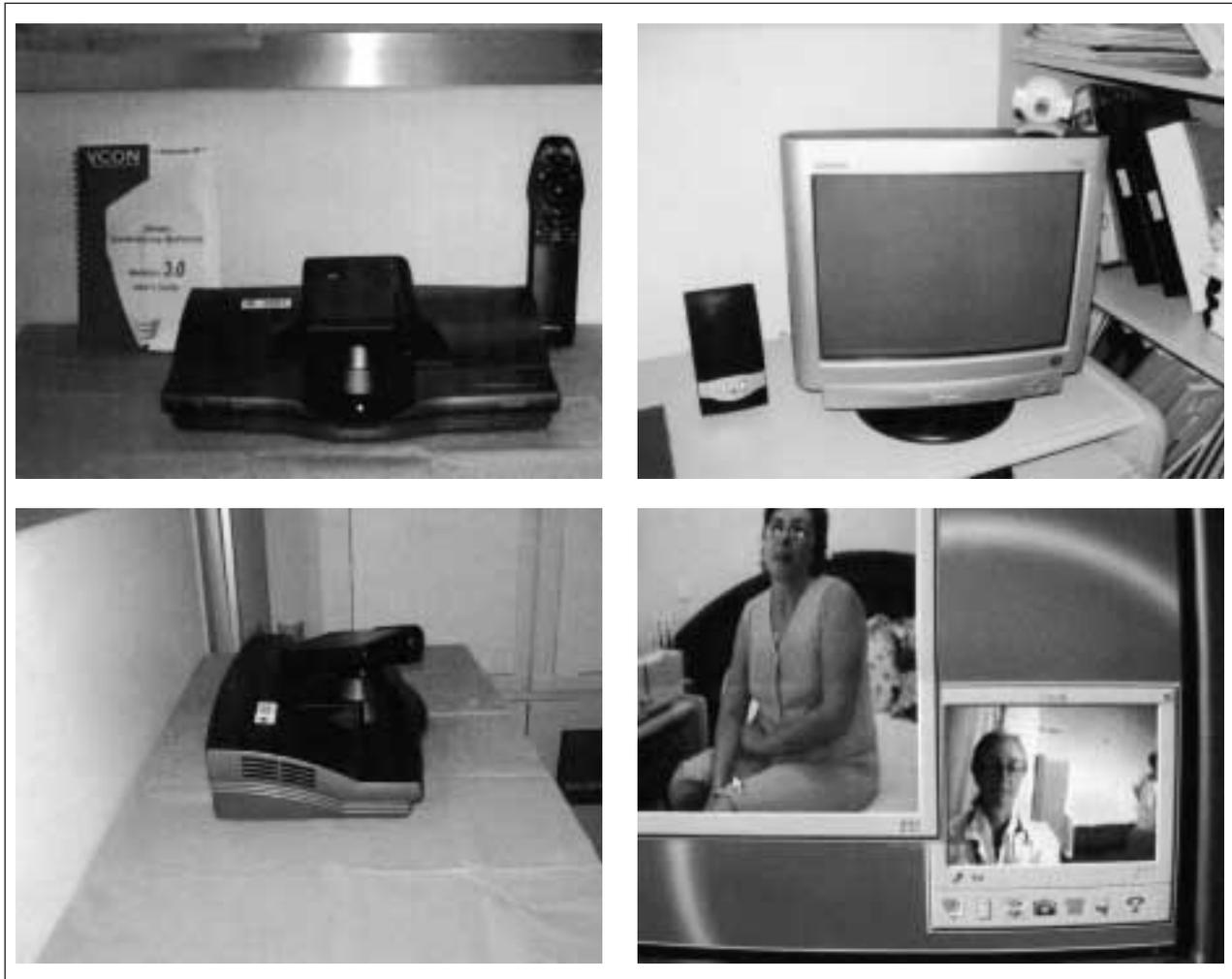
Fig. 1.— Equipment at the patient's home: videoconference equipment with a camera remotely controlled from the hospital. Equipment at the hospital: computer, videoconference card, and webcam.
