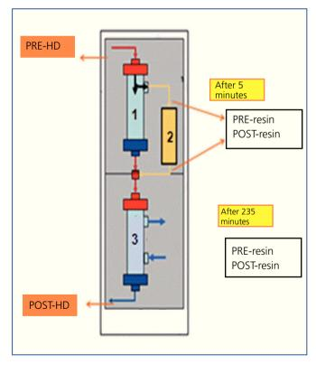
**Figure 1.** Haemodiafiltration diagram with ultrafiltrate regeneration through adsorption in resin.
